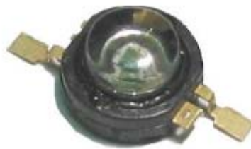
Figura 7.11. Led de potencia luxeon emitter.
