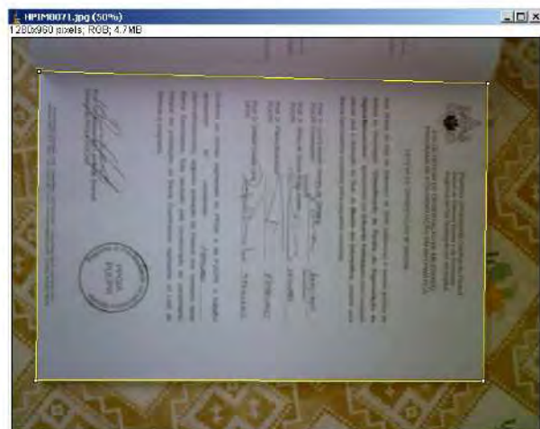
Figure 07 - Document image with edges (in yellow) automatically detected by PhotoDoc
