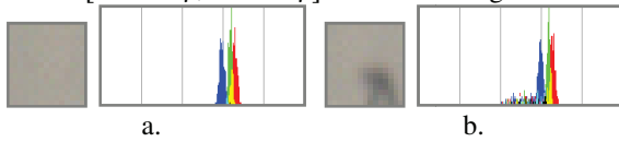
Figure 1. Small blocks and their histograms: Background block (a); Block with "A" letter (b)
