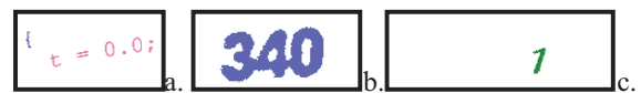
Figure 15. Line missing examples: lines with punctuation marks and a single character (a); undersegmented binarization (b); page number with a single digit (c)
