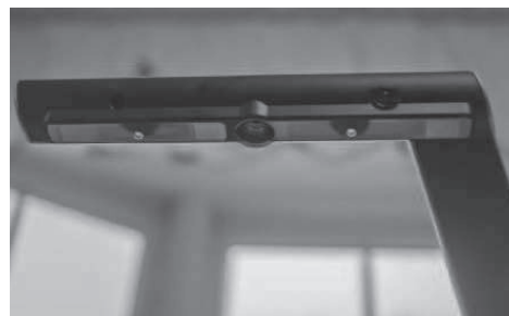
Fig. 4. Detail of the camera and illumination set-up of the “3D-scanner”
