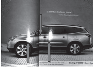
Fig. 1. Photo of a two page magazine printed on glossy paper with specular noises
