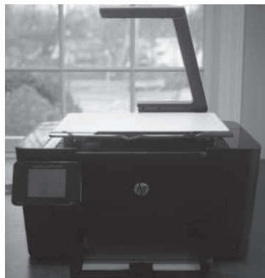
Fig. 3. Photo of the HP TopShot laser printer with “3D-scanner”
