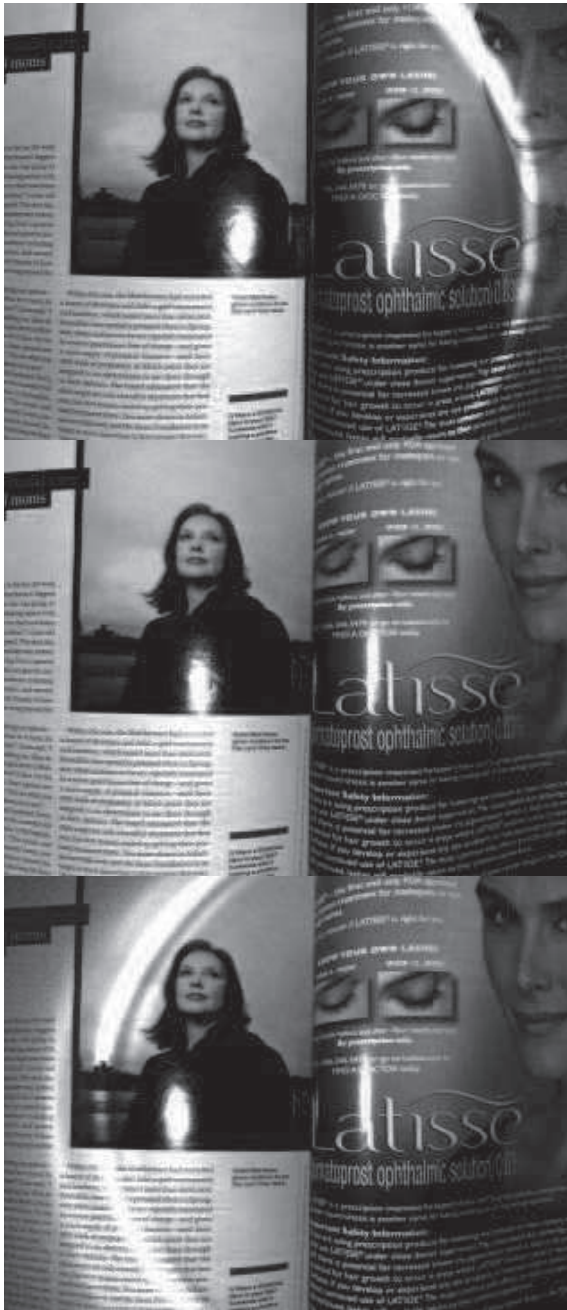
Figure 4 – Document photographed with the second platform. Top: Right lamp only. Center: Central lamp only. Bottom: Left lamp only.
