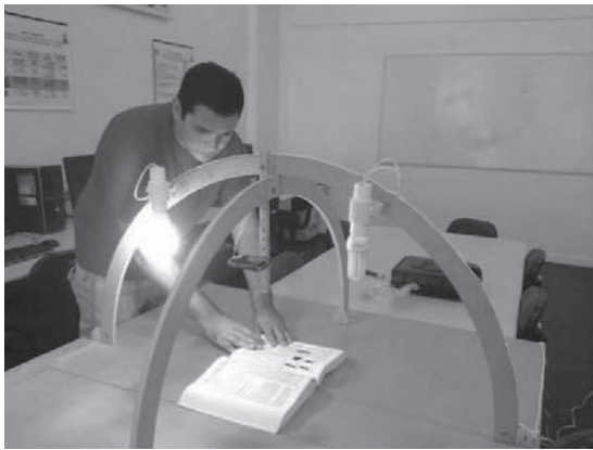
Figure 2 – Digitization platform with two light sources and portable digital camera ( UFPE-Planetarium ).
