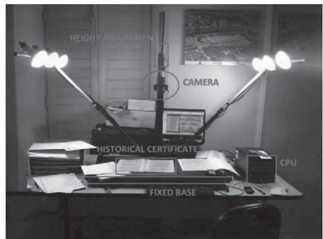
Figure 1 – Digitalization platform used by the Mormon Church to acquire the images of the death certificates in Pernambuco (Brazil).
