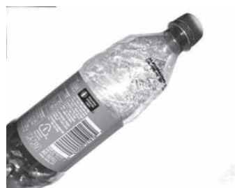
Fig. 13. Image of Figure 1 with the specular noise removed by the application of the algorithm proposed in the areas affected by the specular noise only
