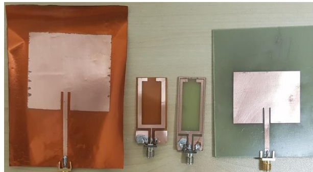
Figure 8.1: Comparative Size of Antennas for FR4 and Pyralux Polyimide
