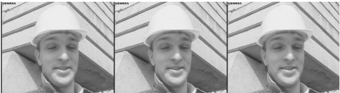
(e) 3D RDCT (PSNR=36.7865, MSSIM = 0.9352), (f) 3D MRDCT (PSNR=36.5764, MSSIM = 0.9280), (g) BAS-2008 (PSNR=37.0146, MSSIM = 0.9378)
